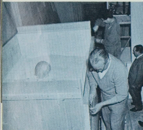
The priceless statue was packed in a heavy wooden case and cushioned with millions of tiny polystyrene beads.
