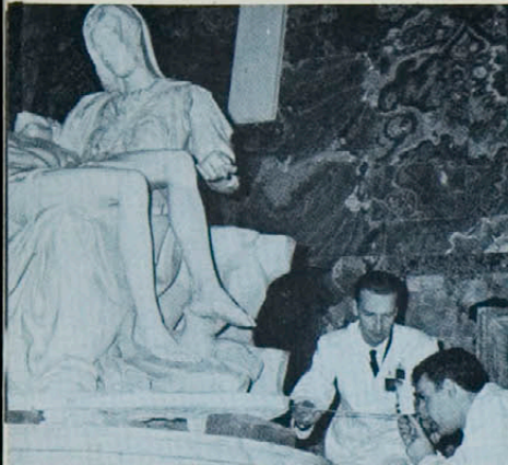
Technicians X-rayed the statue before it was moved from its pedestal in the Basilica.
